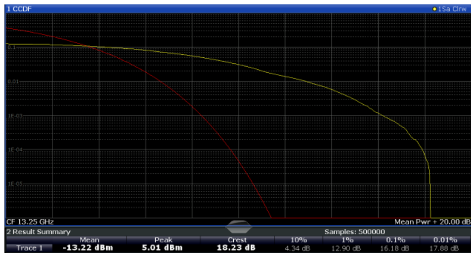
Fig. 3-22: CCDF measurement results for TD-SCDMA BTS measurements
