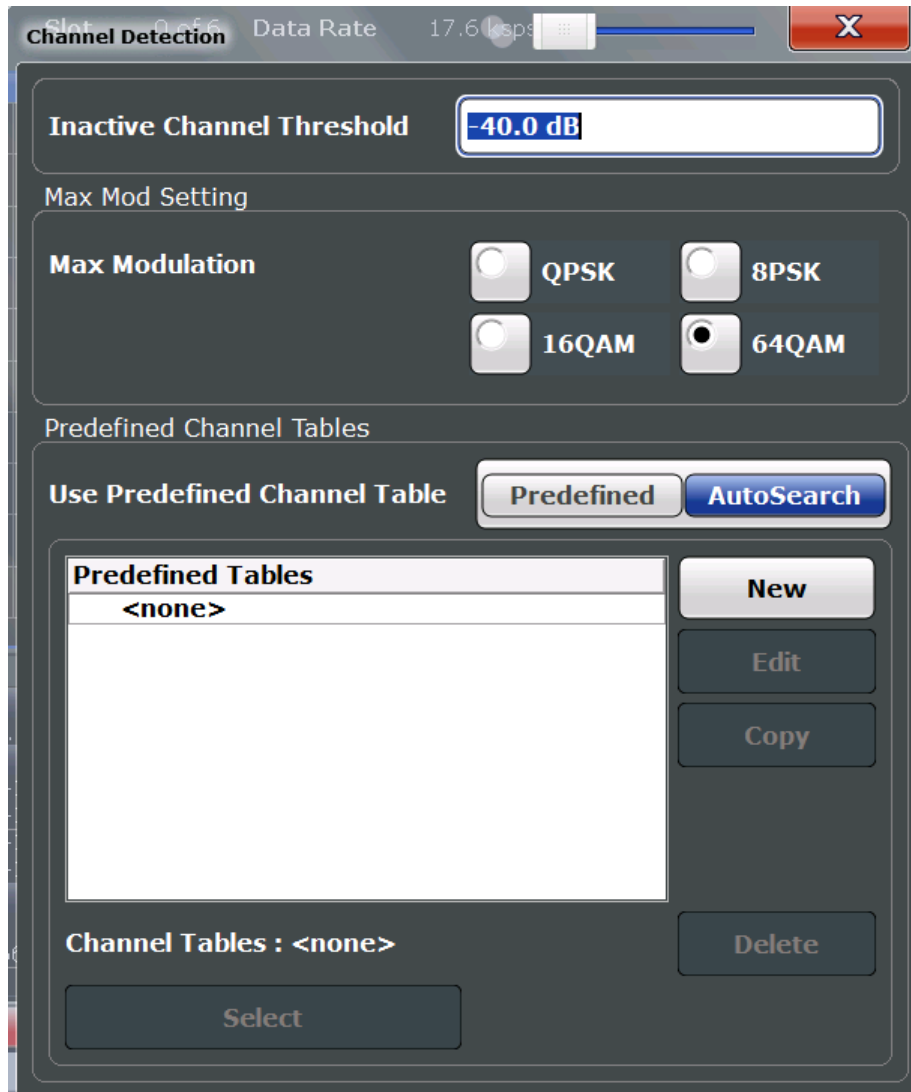
Fig. 6-1: Channel detection configuration for TD-SCDMA BTS application
